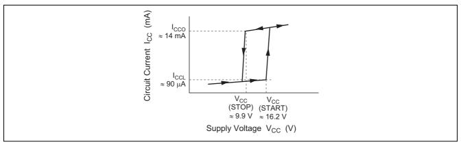
Figure 1 Circuit Current vs. Supply Voltage
