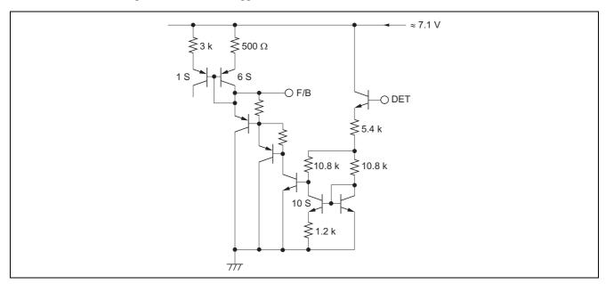
Figure 15 Equivalent Circuit Diagram of Voltage Detector
