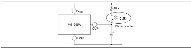
Figure 26 Peripheral Circuit of OVP Terminal
