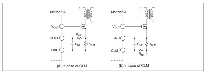
Figure 10 How to Connect Current Limit Circuit
