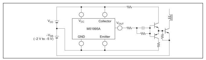
Figure 45 Driver Circuit Diagram (1) for Bipolar Transistor
