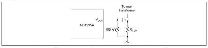
Figure 38 Circuit Diagram to Prevent the MOS FET Gate Potential Rising
