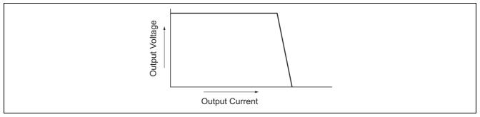
Figure 32 Over Current Limiting Curve on Feed Forward System
