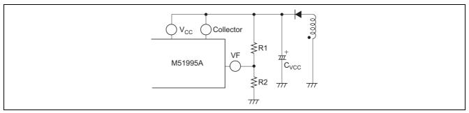
Figure 36 Circuit Diagram to make Knee Point Low on Fly Back System
