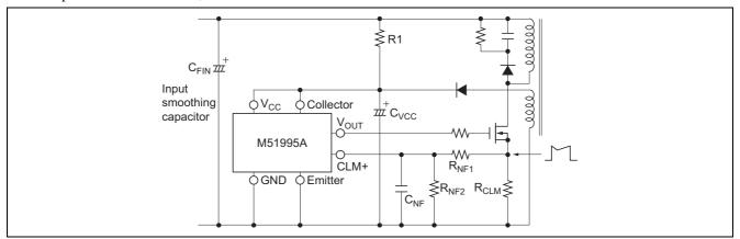
Figure 29 Peripheral Circuit Diagram of CLM+ Terminal
