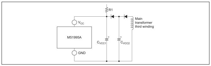
Figure 25 DC Source Circuit for Stable Start-up
