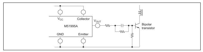
Figure 46 Driver Circuit Diagram (2) for Bipolar Transistor
