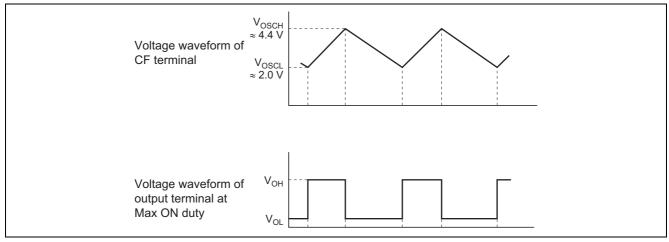
Figure 4 OSC Waveform with Operation of Intermittent and OSC Control Circuit Operation
