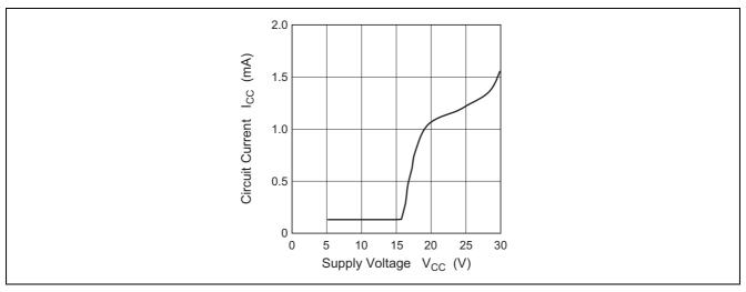
Figure 14 I<sub>CC</sub> vs. V<sub>CC</sub> in Timer-off Duration of Intermittent Action Circuit
