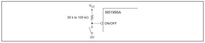
Figure 18 Connecting of ON/OFF Terminal
