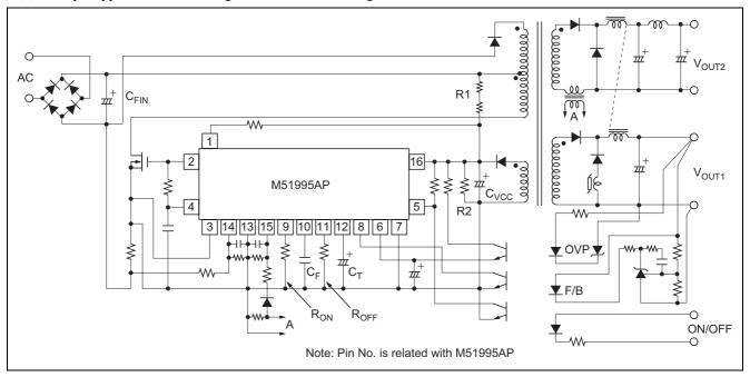
(2) Example application circuit diagram of fly-back regulator
