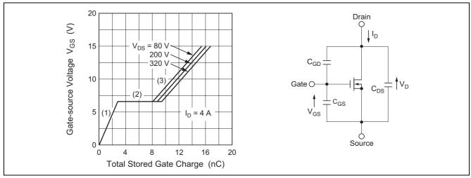
Figure 39 The Relation between Applied Gate-Source Voltage and Stored Gate Charge
