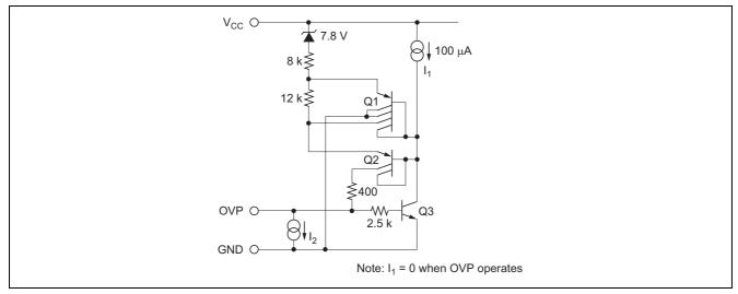
Figure 20 Detail Diagram of OVP Circuit
