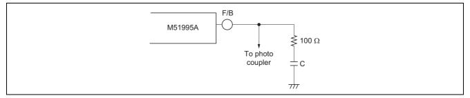
Figure 43 How to Get the Narrow Pulse Width During the Start of Operation
