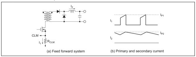
Figure 31 Primary and Secondary Current Waveforms Under the Current Limiting Operation
