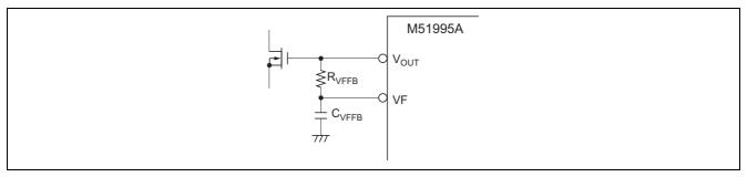
Figure 33 Feed Back Loop through Low Pass Filter from Vout to VF Terminal
