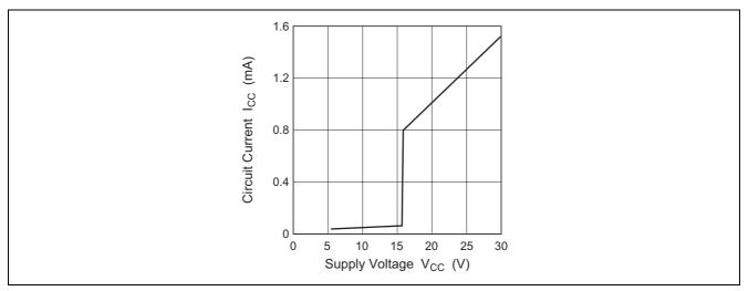
Figure 19 I<sub>CC</sub> vs. V<sub>CC</sub> in OFF State
