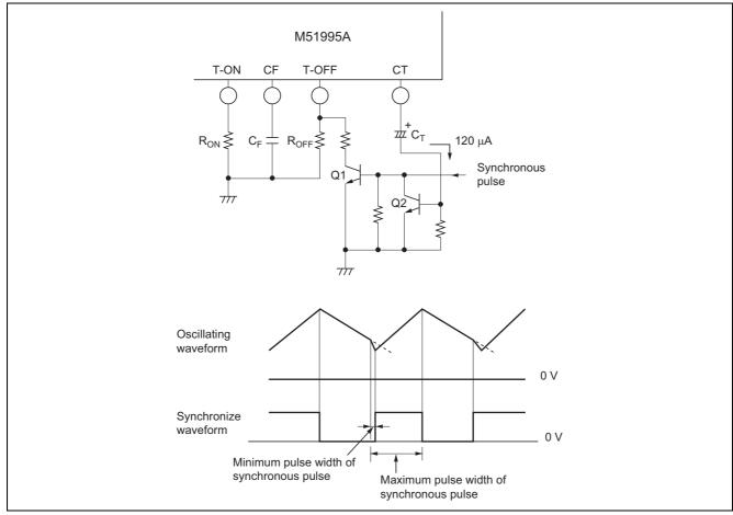
Figure 44 How to Synchronize with External Circuit
