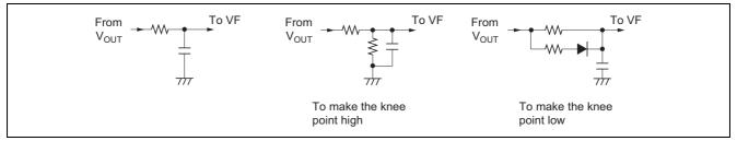
Figure 34 How to Control the Knee Point
