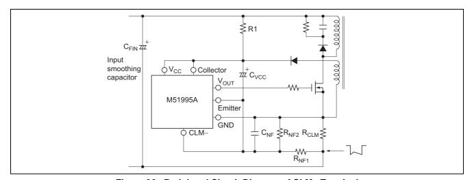
Figure 30 Peripheral Circuit Diagram of CLM- Terminal
