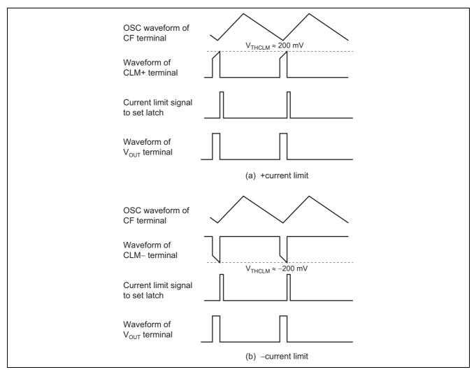
Figure 9 Operating Waveforms of Current Limiting Circuit
