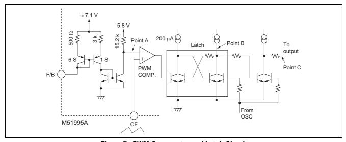
Figure 7 PWM Comparator and Latch Circuit
