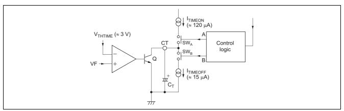
Figure 12 Block Diagram of Intermittent Action Circuit
