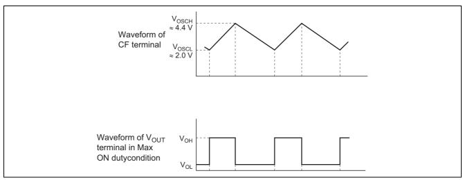
Figure 2 OSC Waveform at Normal Condition (no-operation of intermittent action and OSC control circuit)
