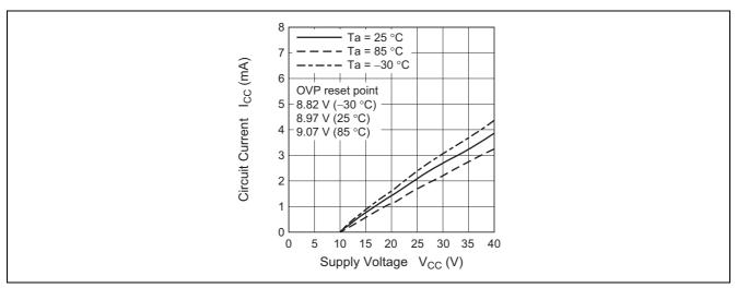
Figure 21 Circuit Current vs. Supply Voltage (OVP Operation)
