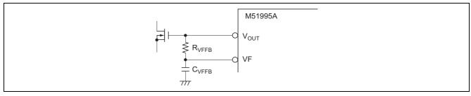
Figure 6 Feedback Loop with Low Pass Filter from Output to VF Terminal
