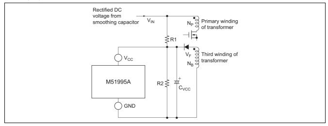
Figure 23 Start-up Circuit Diagram (when it is not necessary to set the start and stop input voltage)
