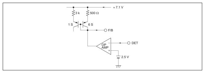
Figure 16 Equivalent Circuit Diagram of Voltage Detector
