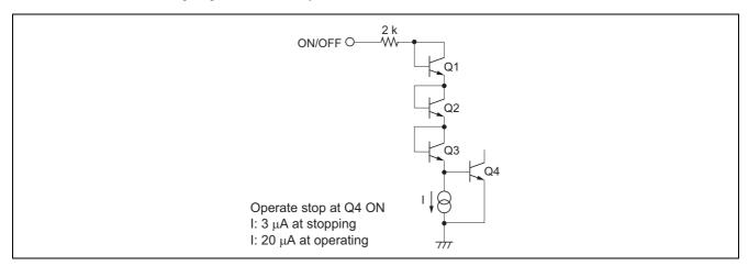
Figure 17 ON/OFF Circuit
