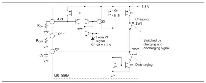
Figure 3 Schematic Diagram of Charging and Discharging Control Circuit for OSC Capacitor C<sub>F</sub>
